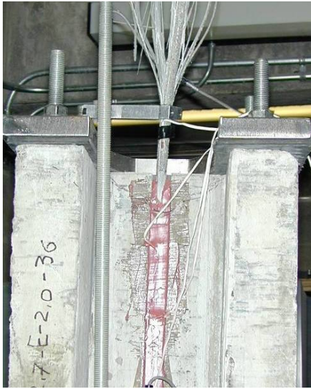
a) Bar rupture for N/G-13-E-2.0-36
