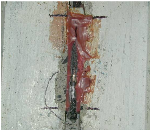
Fig. 6 - Mode of failure for specimens with NSM-GFRP bar and epoxy adhesive.
