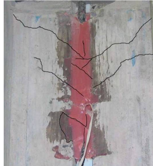
b) Concrete tension failure with epoxy cracking for N/C-10-E-2.0-18
