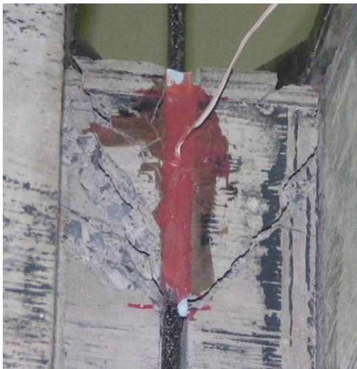
a) Concrete tension failure for N/C-10-E-1.5-12
